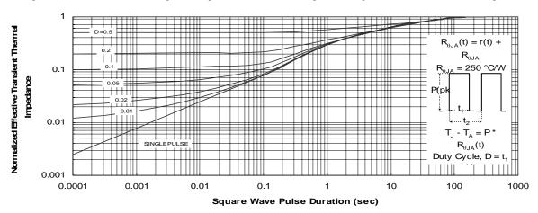
Figure 11. Transient Thermal Response Curve
